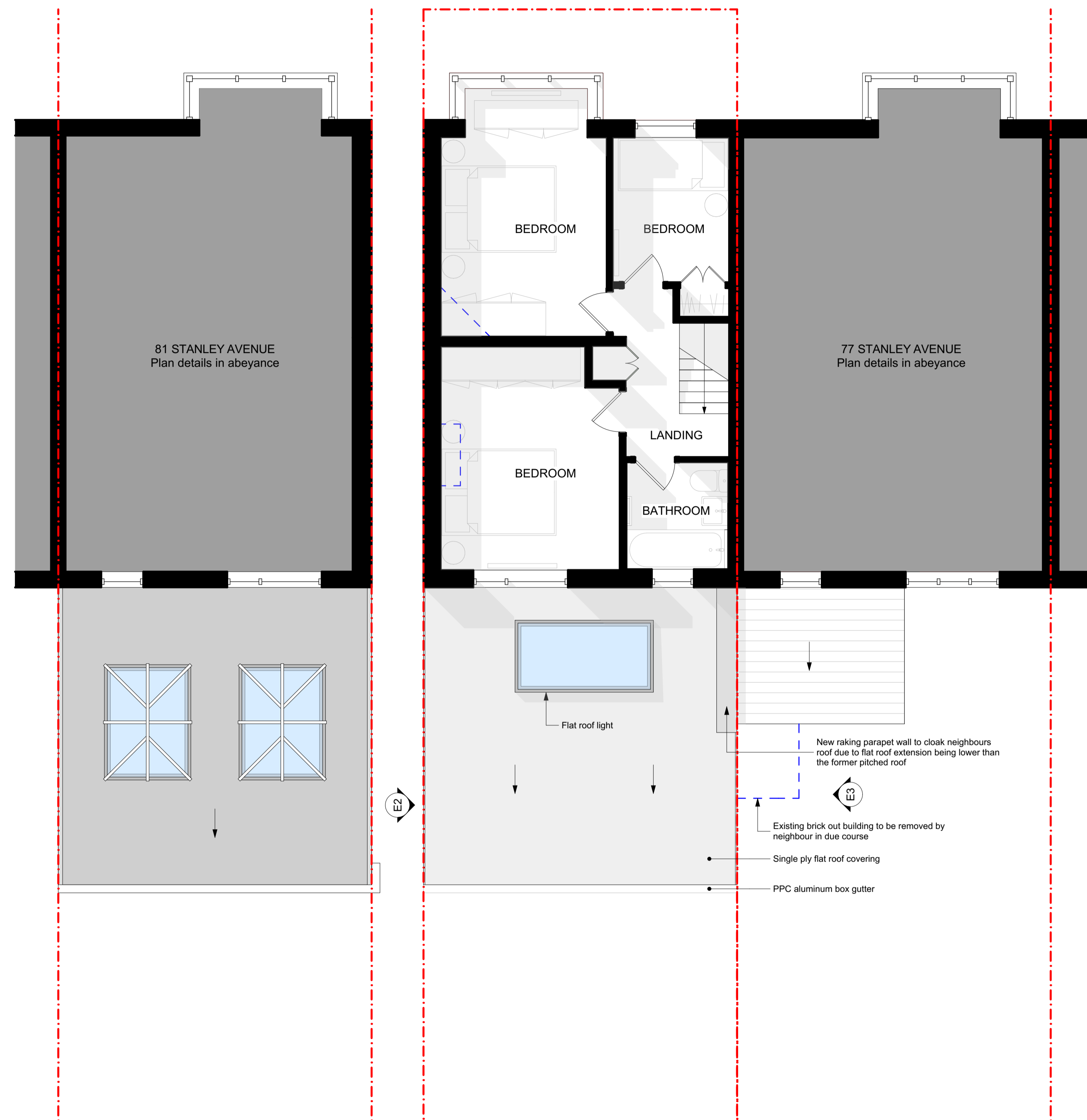
Proposed First Floor Plan 1:50
